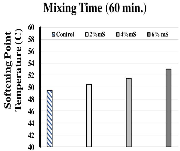
Fig.4: Softening Point of Original Asphalt and mS-Modified asphalt at Mixing Time 60 Minute.
