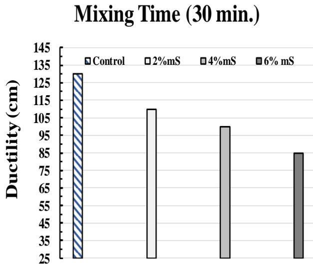
Fig.6: Ductility of Original Asphalt and mS-Modified asphalt at Mixing Time 30 minute.
