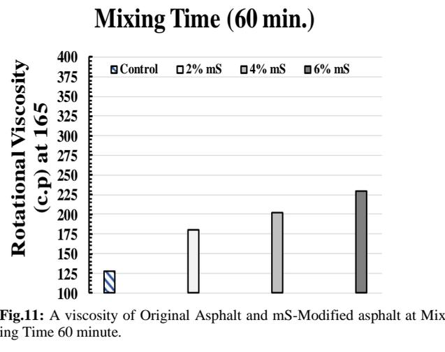
Fig.11: A viscosity of Original Asphalt and mS-Modified asphalt at Mixing Time 60 minute.
