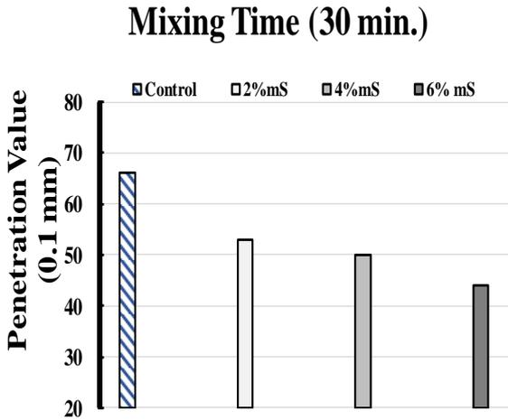
Fig. 1: Penetration Value of Original Asphalt and mS-Modified asphalt at Mixing Time 30 Minute.
