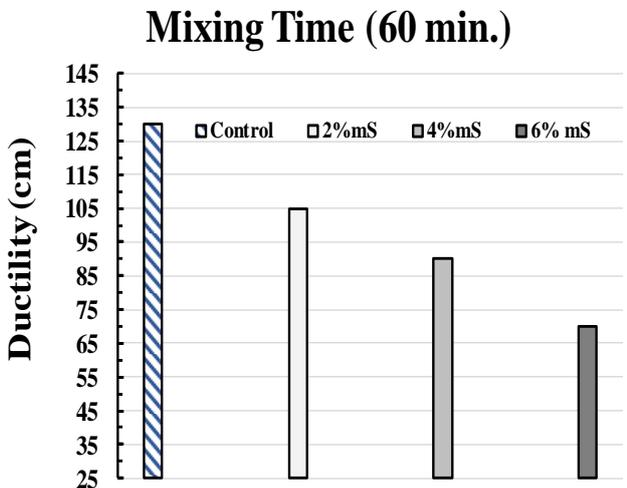
Fig.7: Ductility of Original Asphalt and mS-Modified asphalt at Mixing Time 60 minute.
