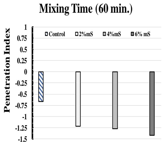
Fig.5: Penetration Index of Original Asphalt and mS-Modified asphalt at Mixing Time 30 & 60 minutes.
