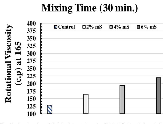
Fig.10: A viscosity of Original Asphalt and mS-Modified asphalt at Mixing Time 30 minute.
