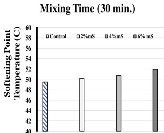
Fig.3: Softening Point of Original Asphalt and mS-Modified asphalt at Mixing Time 30 Minute.
