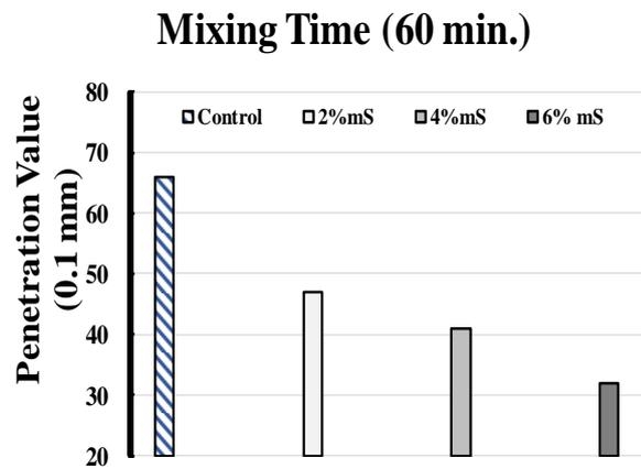
Fig. 2: Penetration Value of Original Asphalt and mS-Modified asphalt at Mixing Time 60 Minute.
