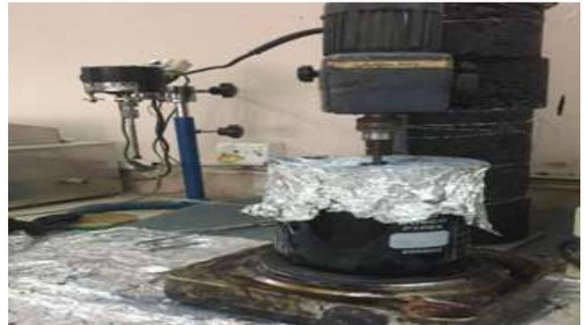
**Plate 1:** Process of mixing of micro silica with asphalt cement under control temperature by using the electronic oven.
