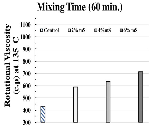
Fig.9: A viscosity of Original Asphalt and mS-Modified asphalt at Mixing Time 60 minute.
