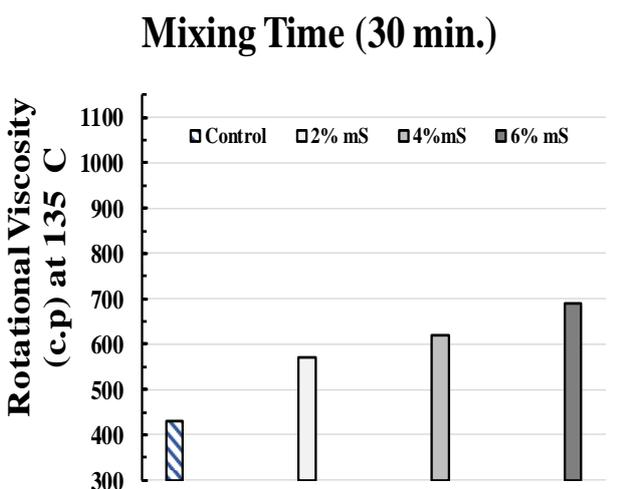
Fig.8: A viscosity of Original Asphalt and mS-Modified asphalt at Mixing Time 30 minute.
