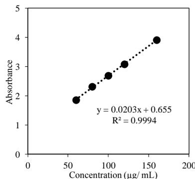
**Fig. 2:** Calibration curve of gallic acid as standard for total phenolic content.
