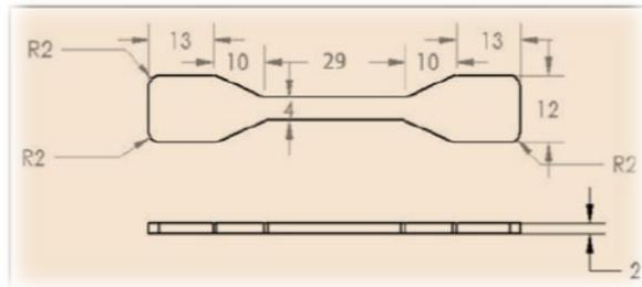
Fig. 1: Sample of injected mould product with dimension (in millimetre)
