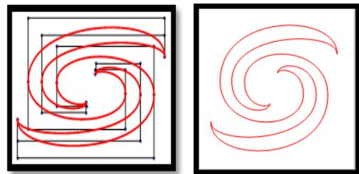
**Fig. 8:** Regenerating Reference Spiral Cubic Curve
