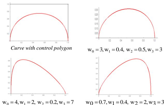
Fig 4: The Cubic Bezier Curve
