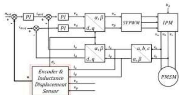
**Figure 4:** SVPWM Simulation block diagram
