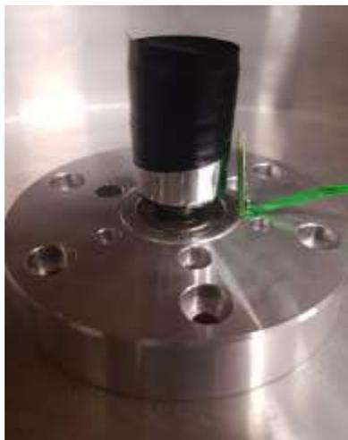
**Figure 2:** Encoder and Inductance Displacement Sensor
