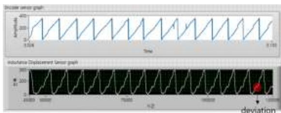
Figure 6: Waveform of Encoder and Inductance Displacement Sensor
