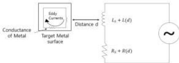
**Figure 1:** Metal Target Modeled as L and R with Circulating Eddy Currents
