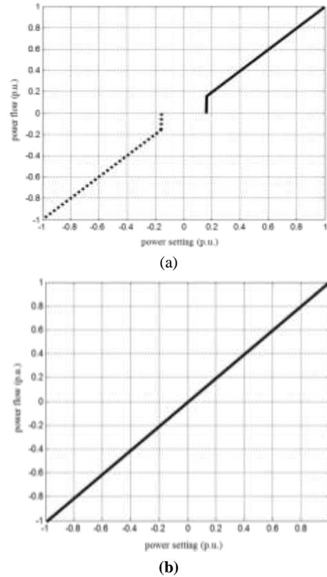
Figure 2: Power flow by power setting of (a) LCC (b) VSC HVDC
