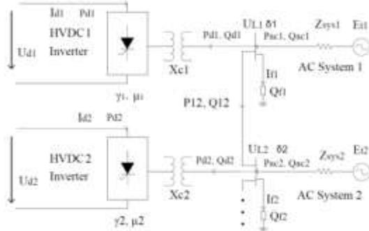
Figure 1: Schematic diagram of the multi-infeed HVDC system
