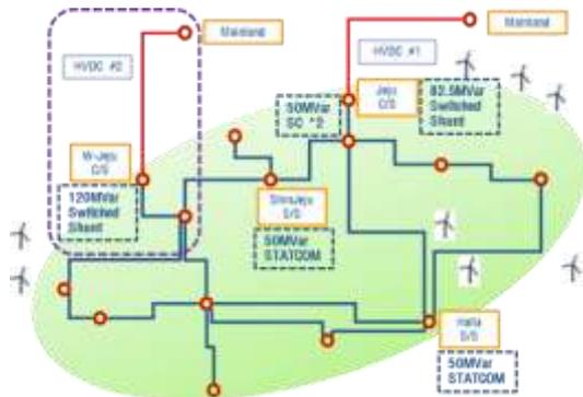
Figure 3: Schematic diagram of Jeju island
