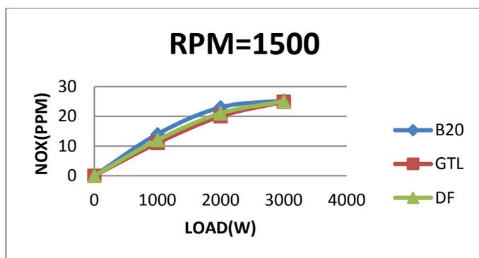
Fig. 7: Variation of NOx with Load
