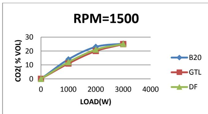
Fig. 8: Variation of CO<sub>2</sub> with Load
