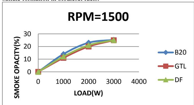
Fig. 9: Variation of Smoke with Load
