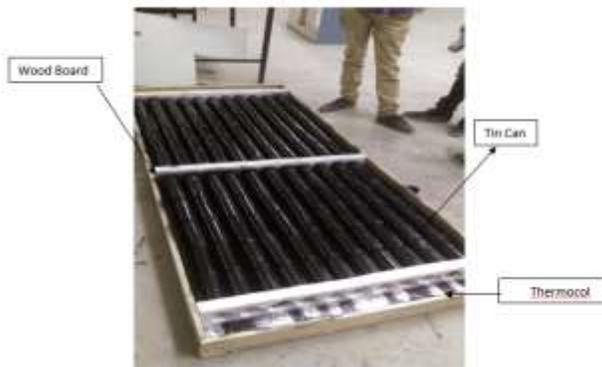
Figure-1: Experimental Set up of Solar Air Heater
