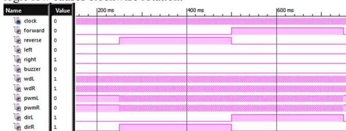
Fig. 6. H-bridge Control Module Simulation
