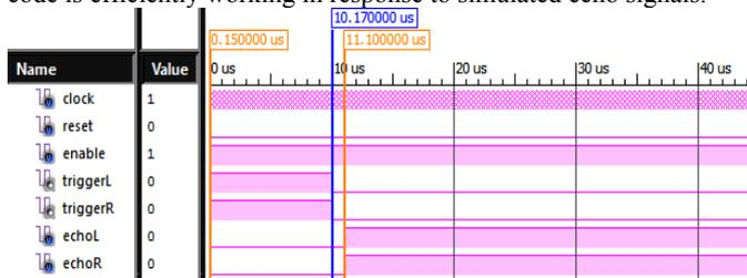
Fig. 5. Ultrasonic sensor transmitter and receiver simulation
