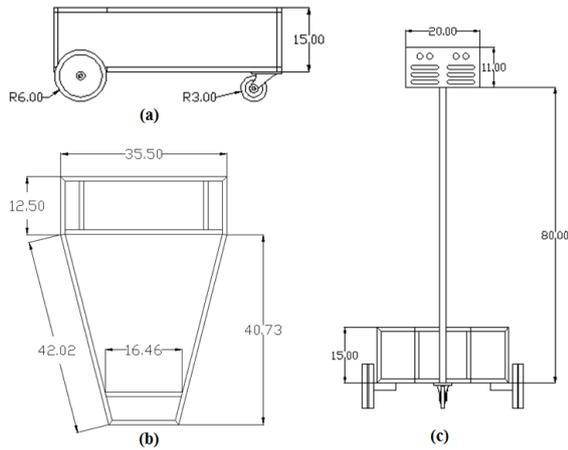
Fig. 1. (a) Side view, (b) Top view and (c) Front view of the cart
