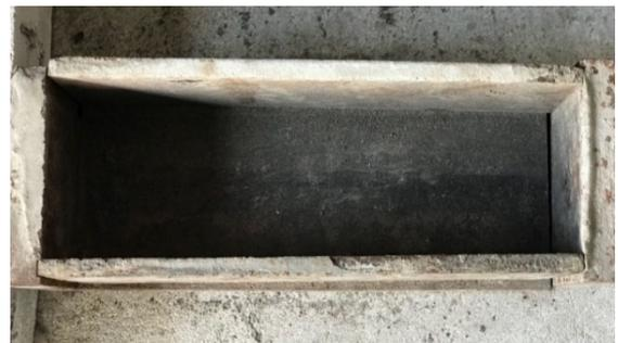
Fig. 6: Prism mould of size 75 x 75 x 285 mm
