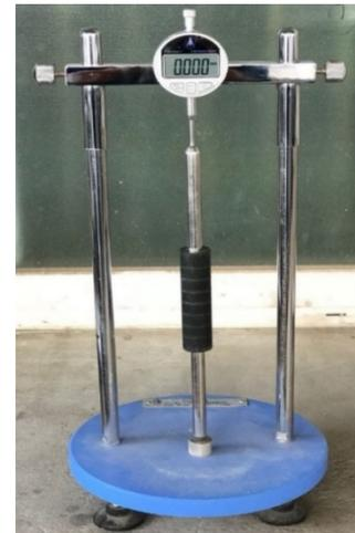
Fig. 7: Length comparator with a standard calibrated rod
