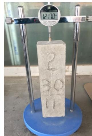
Fig. 8: Digital Length Comparator Apparatus with Specimen for testing
