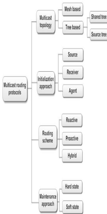
Fig. 1. Classification dimensions of multicast routing protocols
