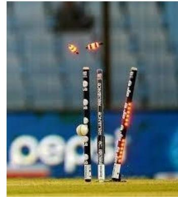
Fig. 5: LED Stumps and Bails.
