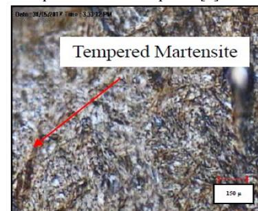
Fig. 6: Structure of tempered martensite
