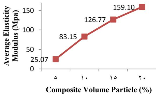
**Fig.6.** Modulus elasticity graphic
