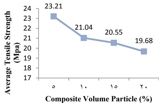
Fig.5. Tensile strength graphic
