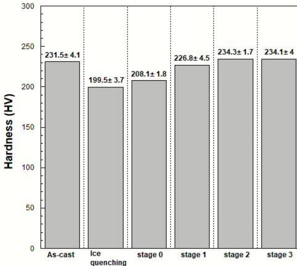
Fig. 3: Hardness change of specimens by cooling stage after simulated porcelain firing
