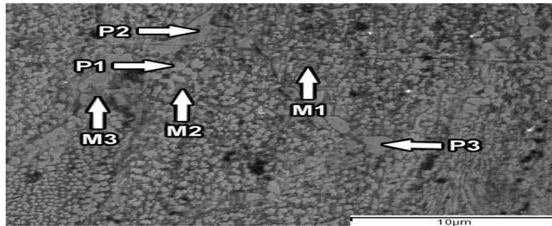
Fig. 8: FE-SEM image of non-heat treated final stage (add-on) specimen (M: Matrix, P: Precipitates)
