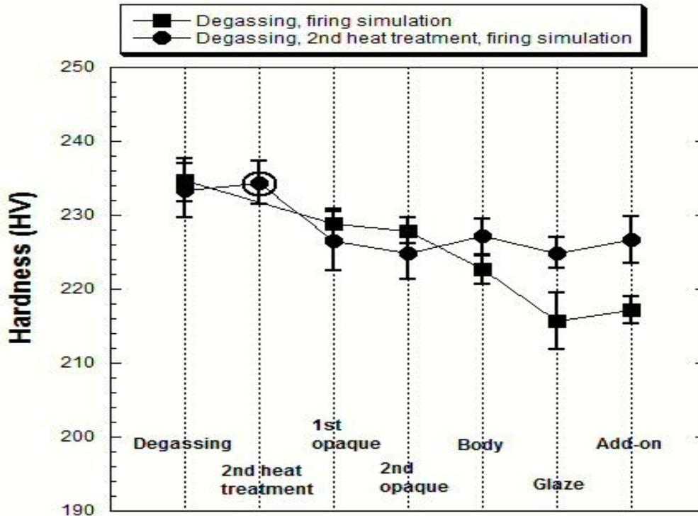
Fig. 4: Change in hardness of the heat treated/non-heat treated specimens during porcelain firing simulation.
