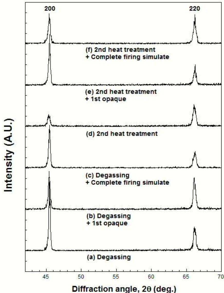
Fig. 7: Change in the XRD pattern during simulated porcelain firing
