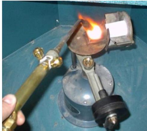
Fig.1: Casting with centrifugal casting machine
