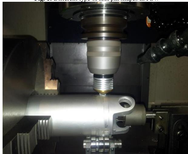
**Fig. 2:** FSW of aluminum tube
