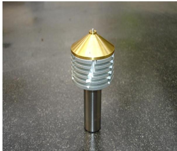
Fig. 3: Tool pin of FSW
