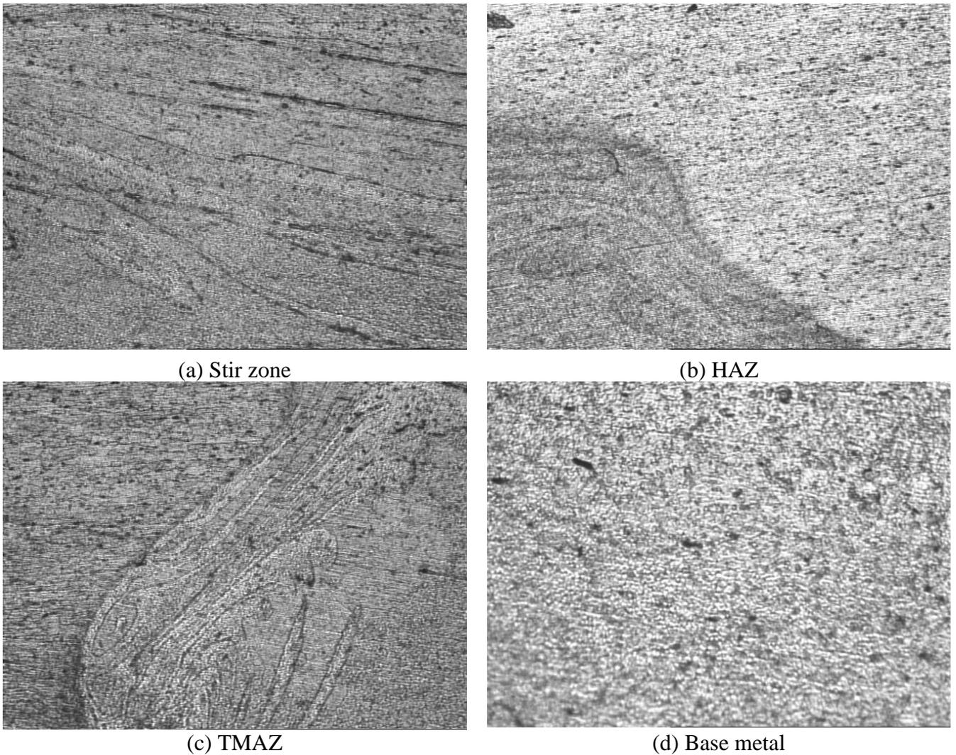
Fig. 10 Cross sectional views of friction stir welded A6061-T6 (×100)
