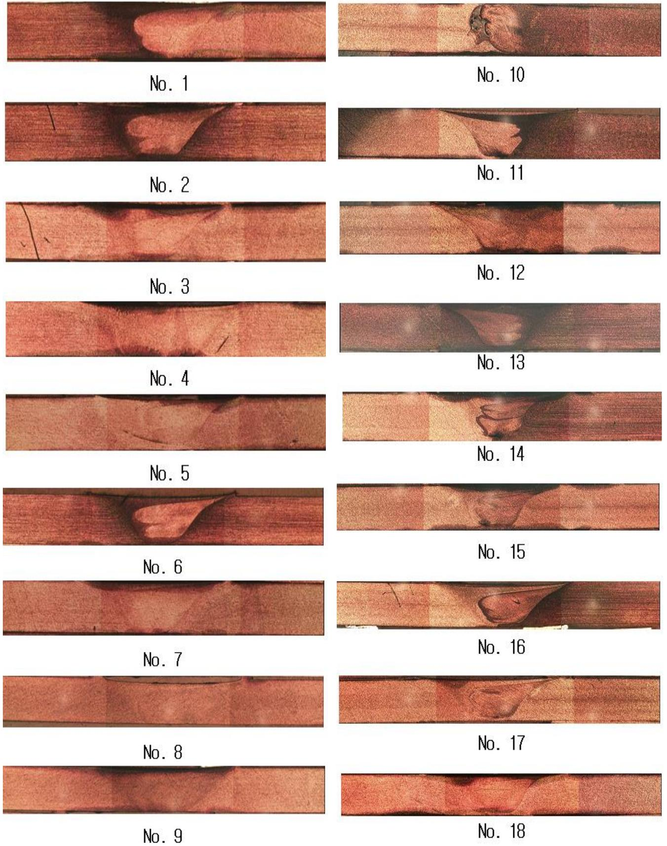
(a) Welding speed low, tool rotation rate(rpm) high
