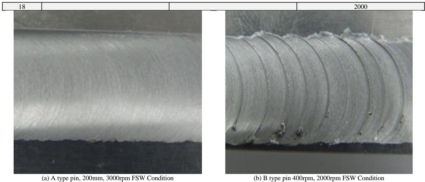
**Fig. 6 :** FSW Results On Different Moving & Tool Rotating Speed
