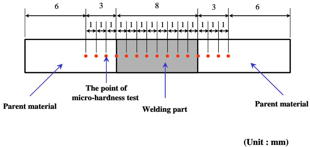
Fig. 5 Measuring Points of micro-vickers hardness
