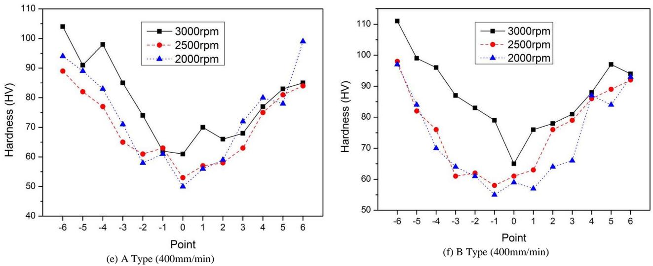
Fig. 9: Result of microhardness measurements
