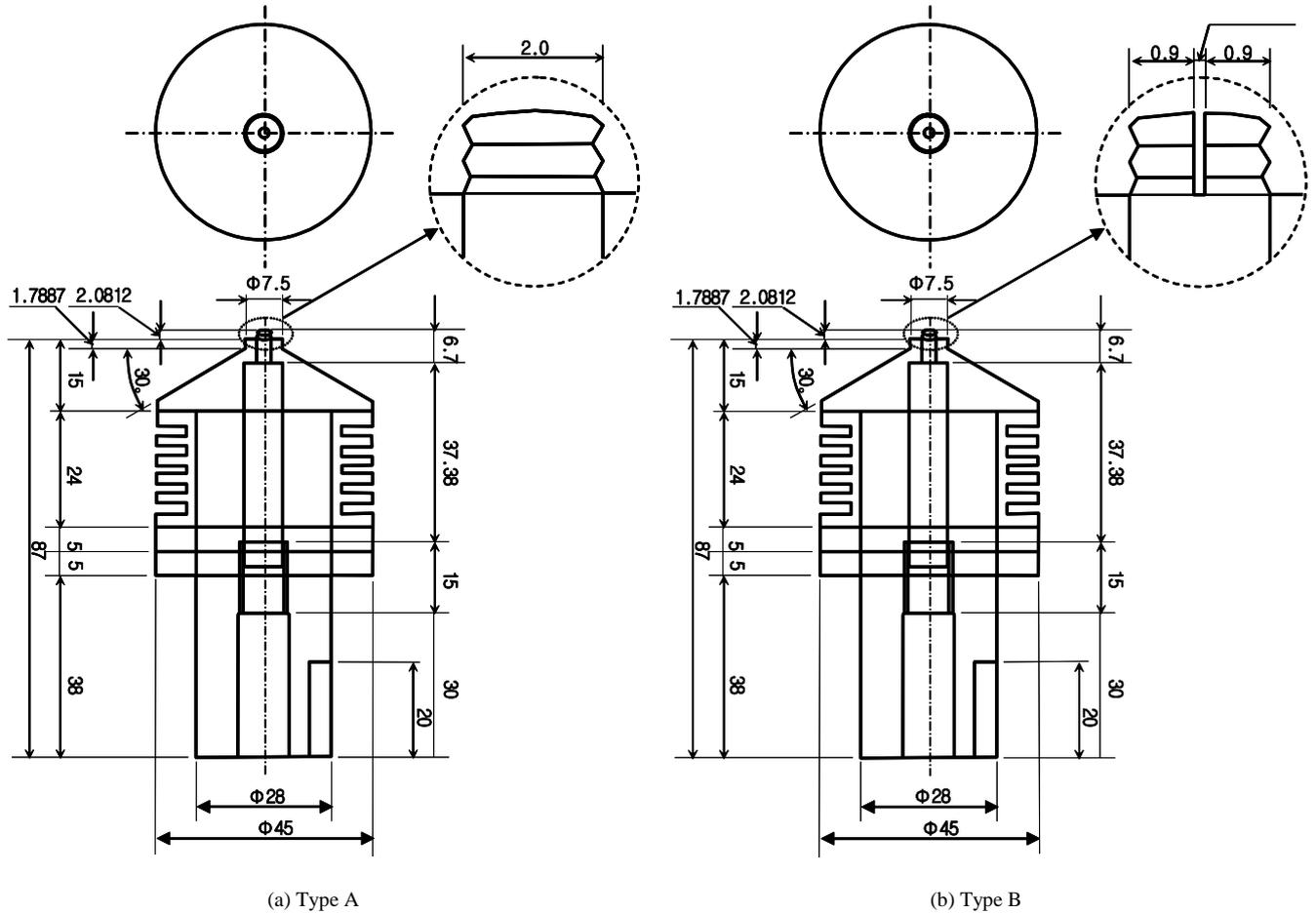
**Fig. 1:** Different type of tool pin shapes in FSW
