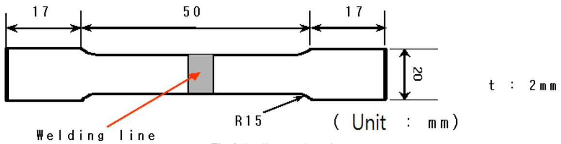
Fig. 4: Tensile strength specimen
