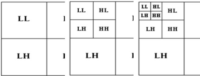
Fig. 7: DWT Decomposed (A) One Level Decomposed. (B) Two Level Decomposed. (C) Three-Level Decomposed.
