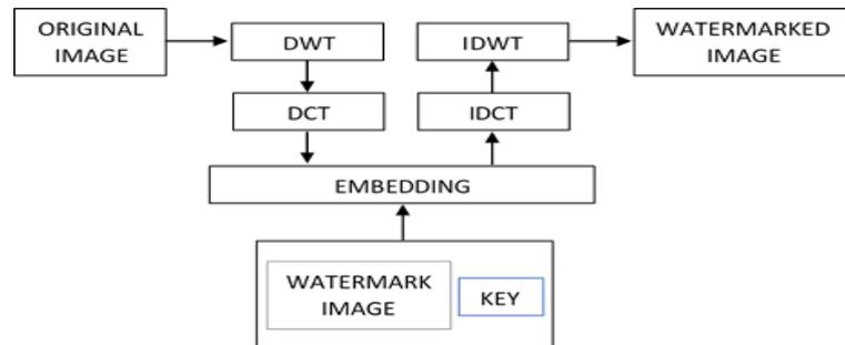
Fig. 2: Digital Watermarking Embedding Process.
