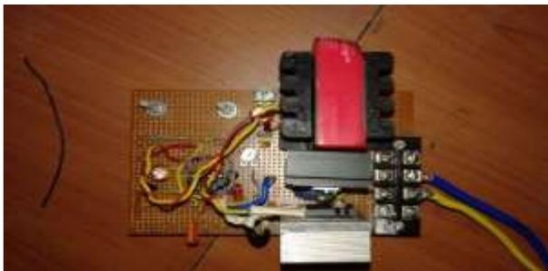
Fig. 1: Buck Converter.
