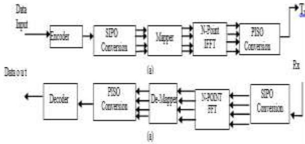
Fig. 1: OFDM Physical Layer System: A) Transmitter, B) Receiver.
