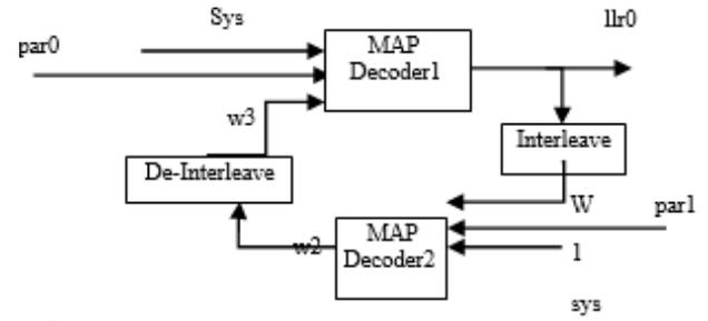
Fig. 3: Block Diagram of Turbo Decoder. Using Map Algorithm.
