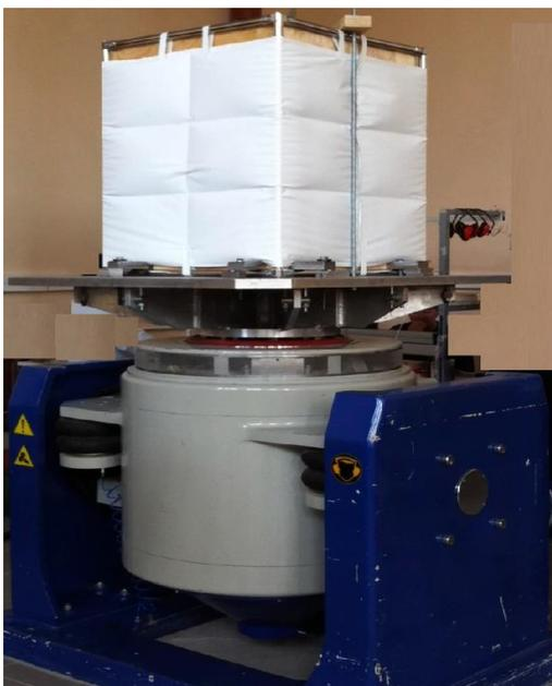
Figure 3 – Experiments with a pneumatic container at shaker table VCB-250-445
