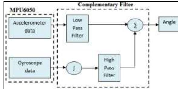
Fig.3: Block diagram of the digital complementary filter
