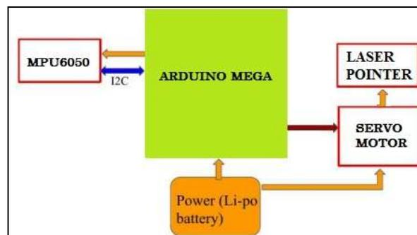
Fig.2: Block diagram of the direction marking system
