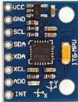
Fig.1: MPU6050 MEMS gyroscope and accelerometer
