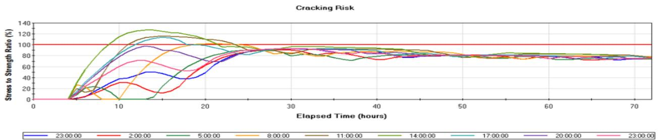
Fig 8 : Cracking Risk Ratio of Concrete Pavement
