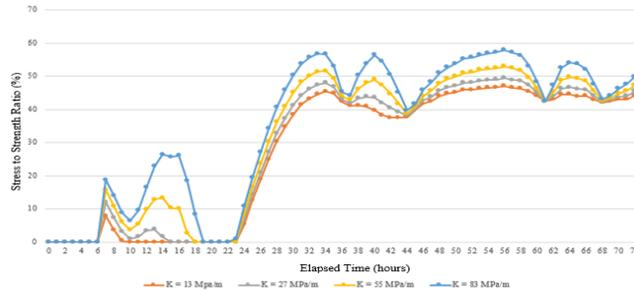
**Fig. 12 :** The relationship between the start time and the stress - strength ratio of concrete (%) for various subgrade reaction of soil (k') nighttime construction, subgrade of soil reaction (k) 25 MPa / m, thick (h) 30 cm and length ( L) 3.44 m
