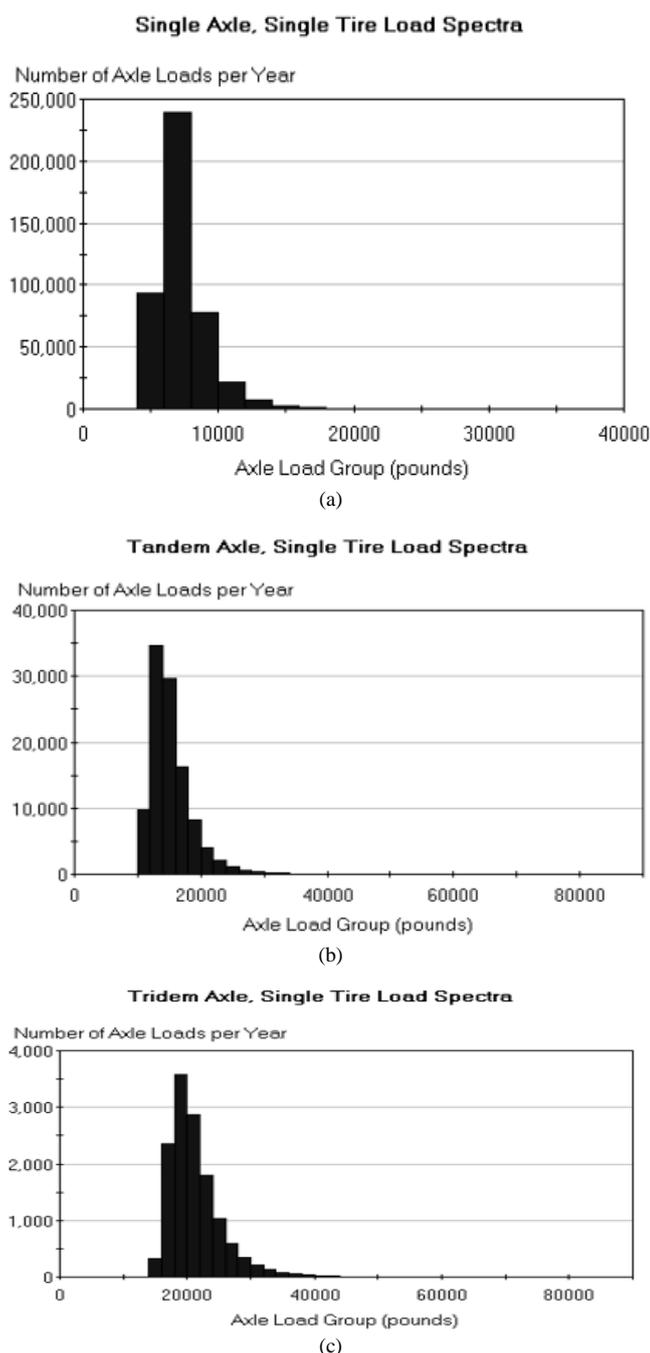
Fig 4: Number of Axle Load Per Year 2014-2016 (a) Single Axle; (b) Tandem Axle; (c) Tridem Axle
