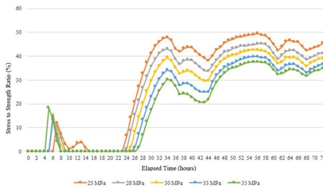
**Fig. 10 :** The relationship between the start time and the stress - strength ratio of concrete (%) for various concrete (fc') and nighttime construction, subgrade of soil reaction (k) 27 MPa / m, thick (h) 25 cm and length (L) 3.44 m
