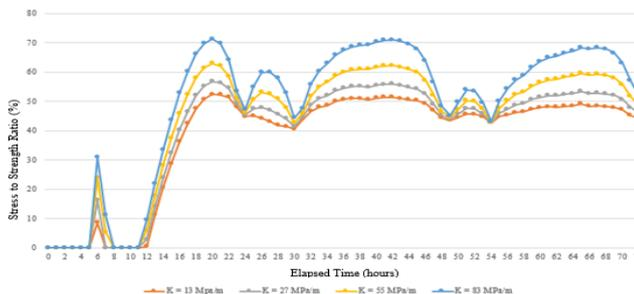
**Fig. 13 :** The relationship between the start time and the stress - strength ratio of concrete (%) for various subgrade reaction soil (k) and daytime construction, subgrade of soil reaction (k) 25 MPa / m, thick (h) 30 cm and length ( L) 3.44 m
