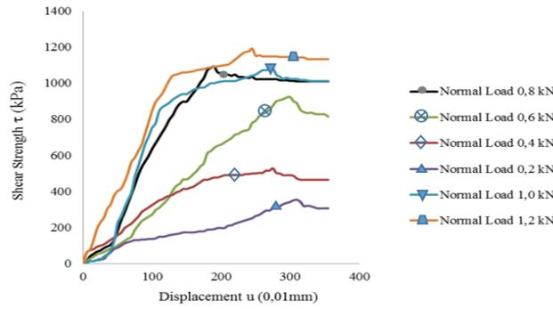
Fig. 4: Shear Strength vs Displacement Residual Condition
