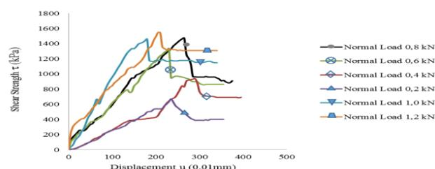
**Fig. 3:** Shear Strength vs Displacement Peak Condition
