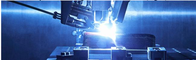
Fig. 3: The Rapid Plasma Deposition process involves metal wire feedstock and argon gas. Image by Norsk Titanium.
