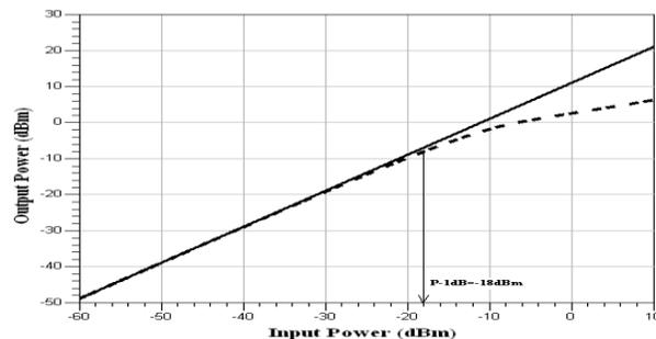
**Fig.4** Input P-1 dB Compression Point
