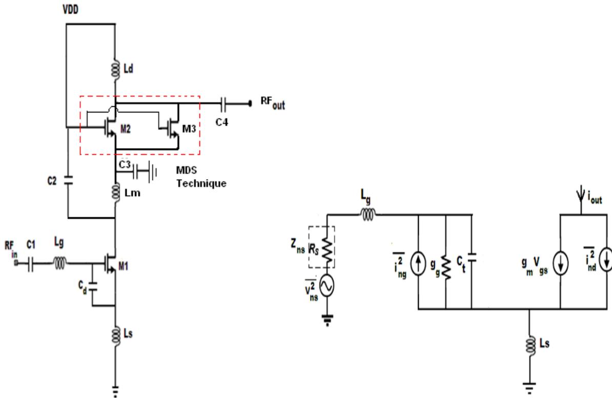
Fig.1(a) Schematic of Current Reuse LNA with MDS (b) Small Signal Equivalent Circuit of input stage
