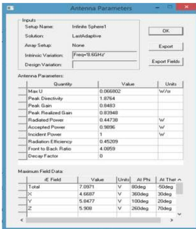
Fig. 9: Antenna parameters at 8.6GHz
