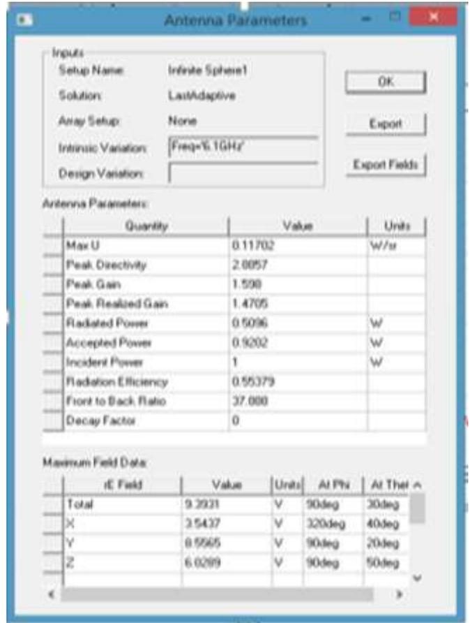
Fig.7: Antenna parameters at 6.1GHz
