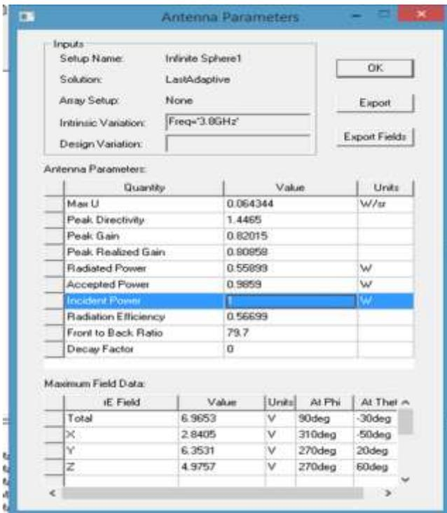
Fig. 6: Antenna parameters at 3.8GHz
