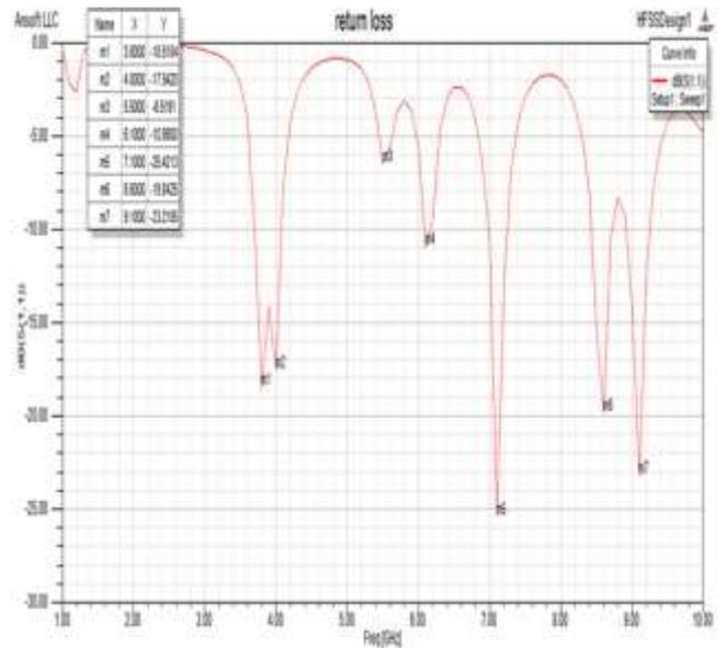
Fig. 3: Return loss VS Frequency plot in HFSS
