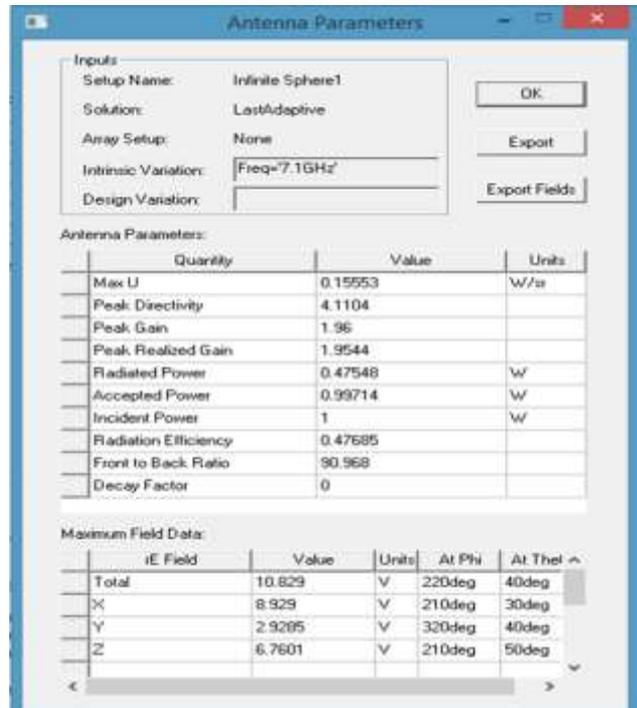
Fig. 8: Antenna parameters at 7.1GHz
