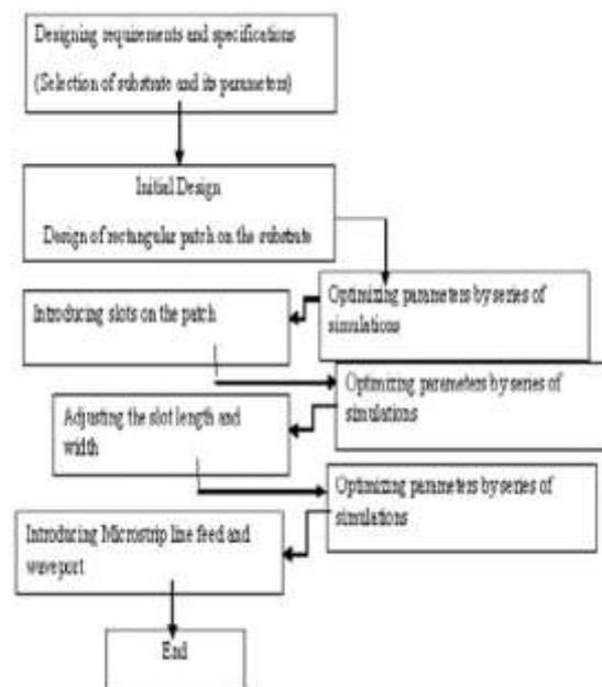
Fig. 1: Design procedure of antenna Figures
