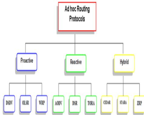
Fig 2: MANETs Routing Protocols
