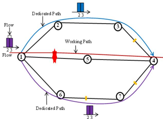
Fig. 1: Power efficient dedicated path protection in elastic optical network.
