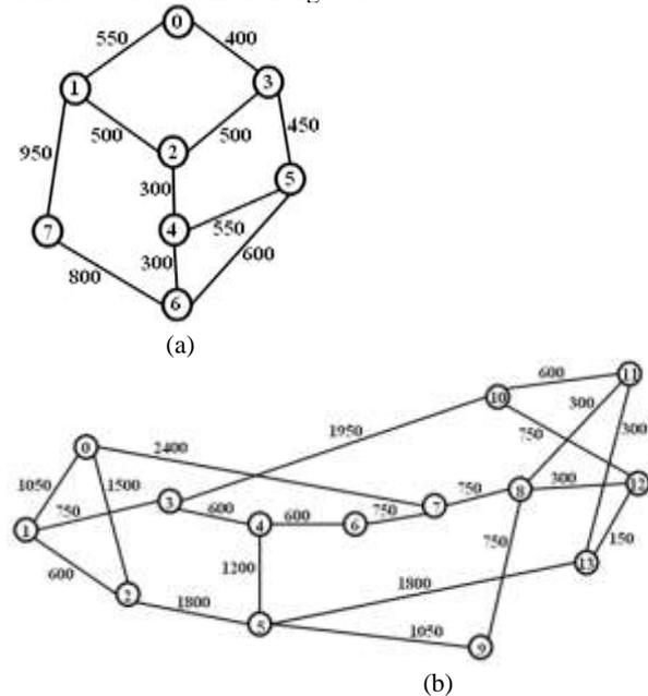
Fig. 4: Network topology used in simulations (a) 8n11s network (b) 14n 21s (NSFNET) network.
