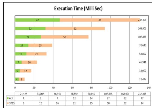
**Fig. 2:** Turnaround time comparison between AES and 3DES
