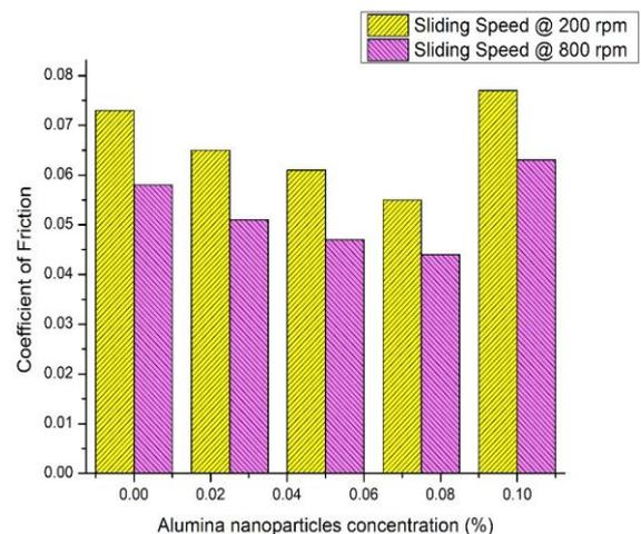
**Figure 2:** Effect of nanoparticles concentration on COF.
