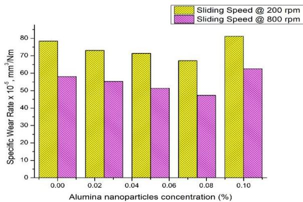
Figure 4: Nanoparticles concentration on specific wear rate.
