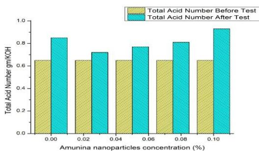
Figure 5: Total acid number with different alumina concentration percentage
