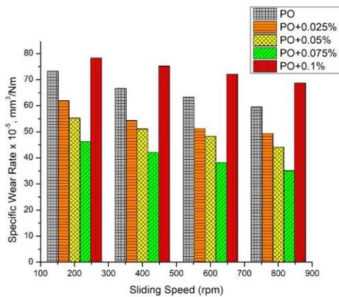
Figure 3: Effect of sliding speed on specific wear rate
