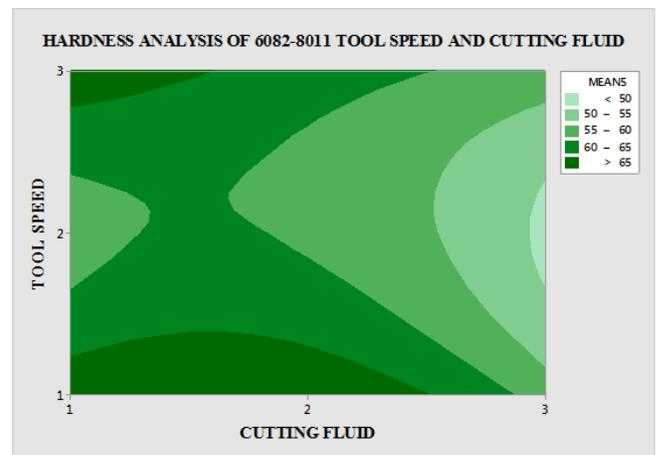
**Fig. 4:** Contour curves of tool speed and cutting fluid
