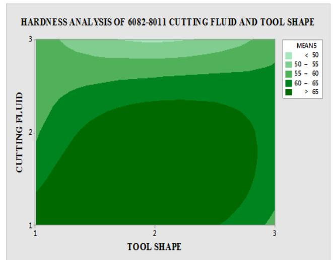
**Fig. 5:** Contour curves of cutting fluid and tool shape
