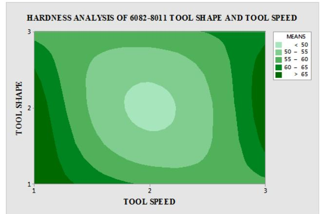
**Fig. 3:** Contour curves of tool shape and tool speed
