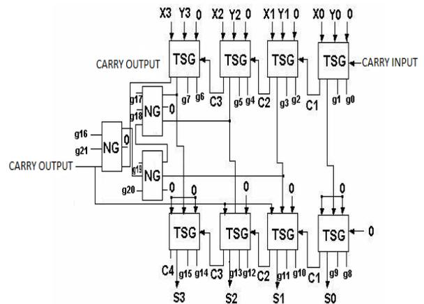
Fig.5: Complimentary implementation of conventional BCD adder
