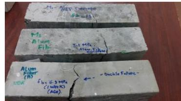
**Fig. 3:** Aluminum strip reinforced concrete Beams after the flexural test.
