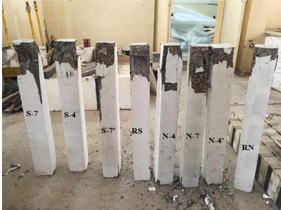
Fig. 3: Failure Pattern
