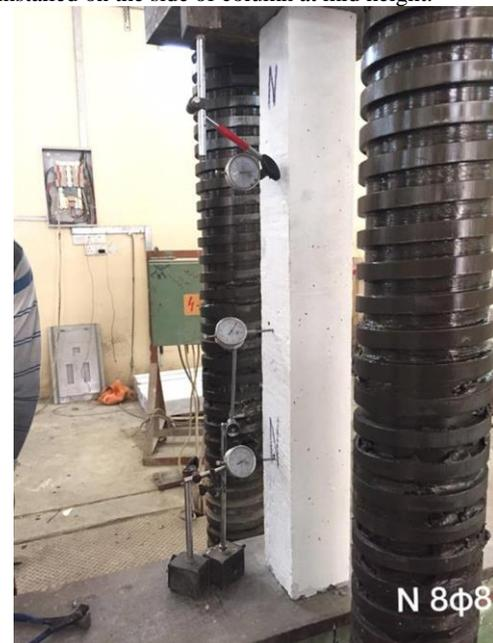
**Fig. 2:** Loading Set up
