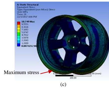
Fig. 6: Stress distribution on (a) aluminium alloy, (b) magnesium alloy and (c) titanium alloy wheels
