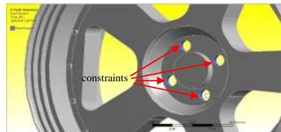
**Fig. 4:** Constraint applied to bolt holes
