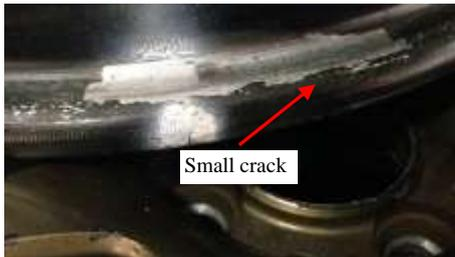
**Fig. 1:** Alloy wheel of a 1200 cc national automobile with a small crack on the outer surface of the rim
