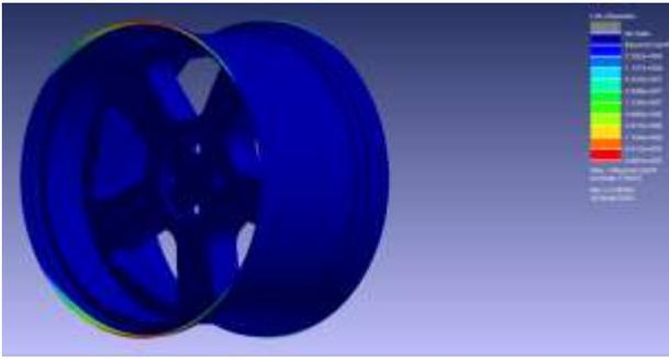
Fig. 8: Number of cycles to failure for magnesium alloy wheel
