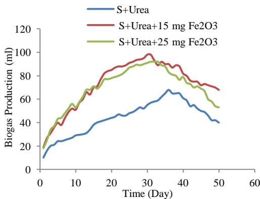
Fig. 3: Variation in daily volume of biogas production with time.
