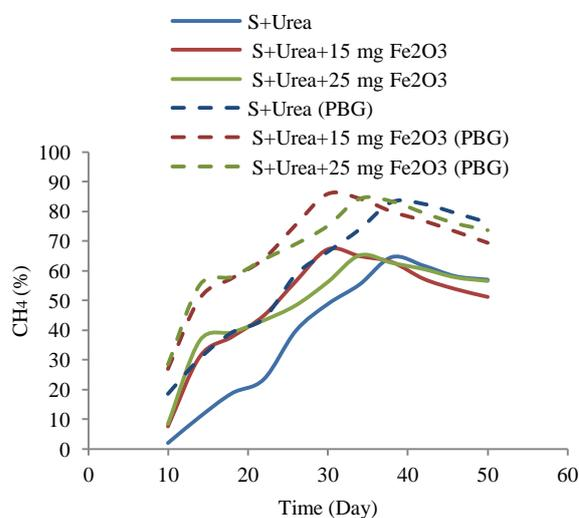
Fig. 2: Variation of  $\text{CH}_4$  content with respect to time.
