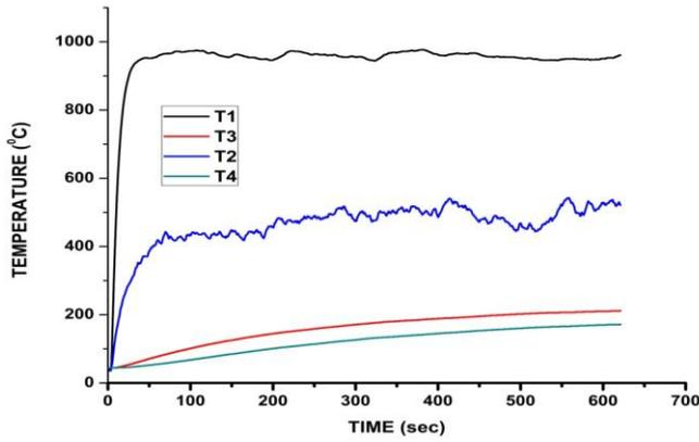
Fig.6(a): Transient temperature distribution at different locations of the burner without secondary aeration.
