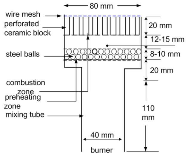
Fig.2: Schematic of the self-aspirated porous surface burner
