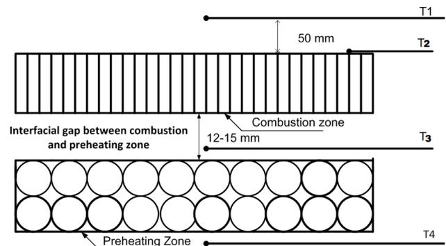
Fig.5: Arrangement of thermocouple to measure temperature at different locations of the burner
