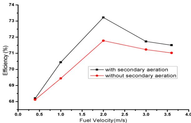
Fig.7: Comparison of thermal efficiency of the burner with and without secondary aeration.
