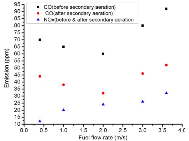
Fig.8: Emission of CO and NOx from the burner with and without secondary aeration
