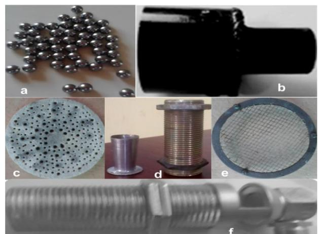
Fig.3: Components of the SAPSB (a) Stainless steel balls (b) burner body (c) perforated ceramic block (d) mixing tube with nozzle (e) wire mesh with supporting frame (f) mixing tube with nozzle and fuel ejector assembly.
