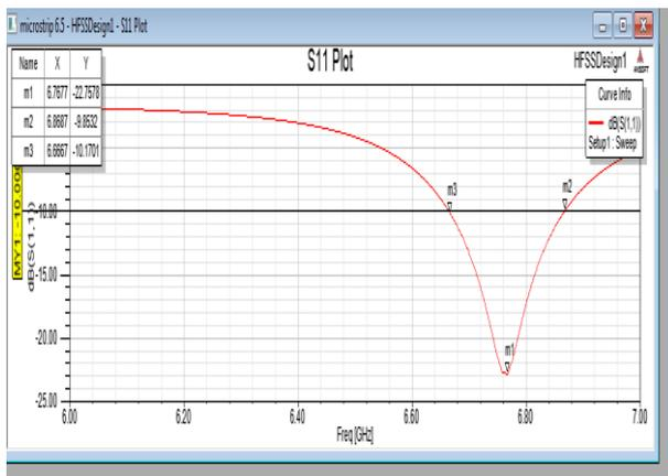
Fig 1: The Return Loss Plot
