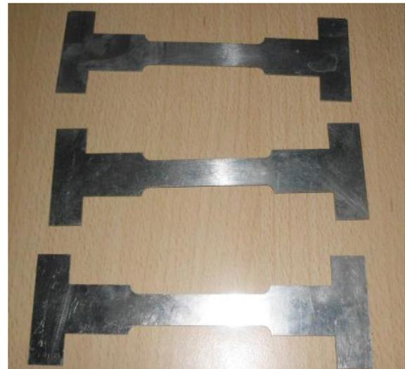
Fig. 7: Tensile Test Specimen Samples.
