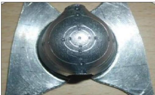
**Fig. 13:** Drawn Specimen (2.0 Mm) with Deformed Circles.
