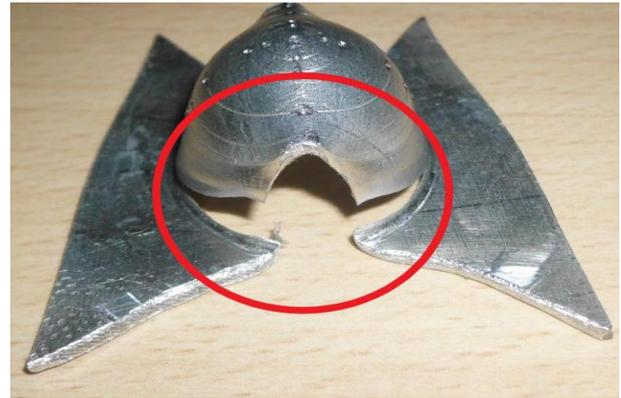
Fig. 17: Tearing, Excessive Thinning, and Earing.
