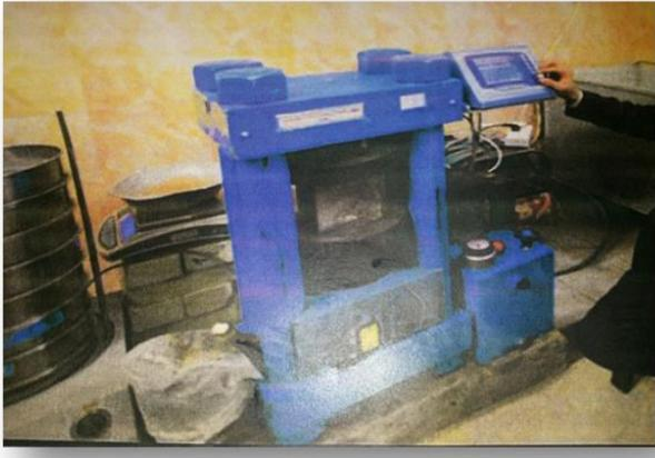
Figure (1) measuring of strength for Thermostone (Durability)
