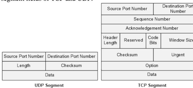
Fig. 1. The Segment Fields of TCP and UDP
