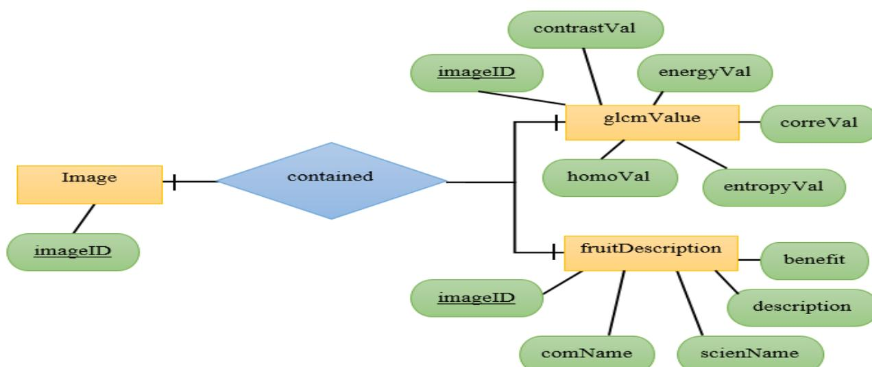
Fig. 5: Entity-relationship Diagram of the System
