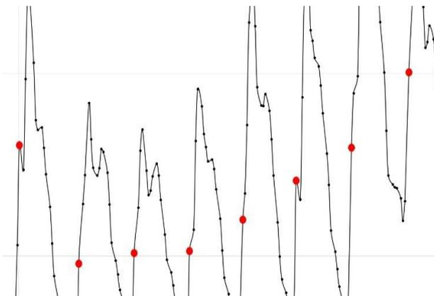
**Fig. 10:** Visual Representation of Striking Hit. Red Spot Indicated the Point of Drum Hit Before It Reached the Actual Peak Acceleration Magnitude.
