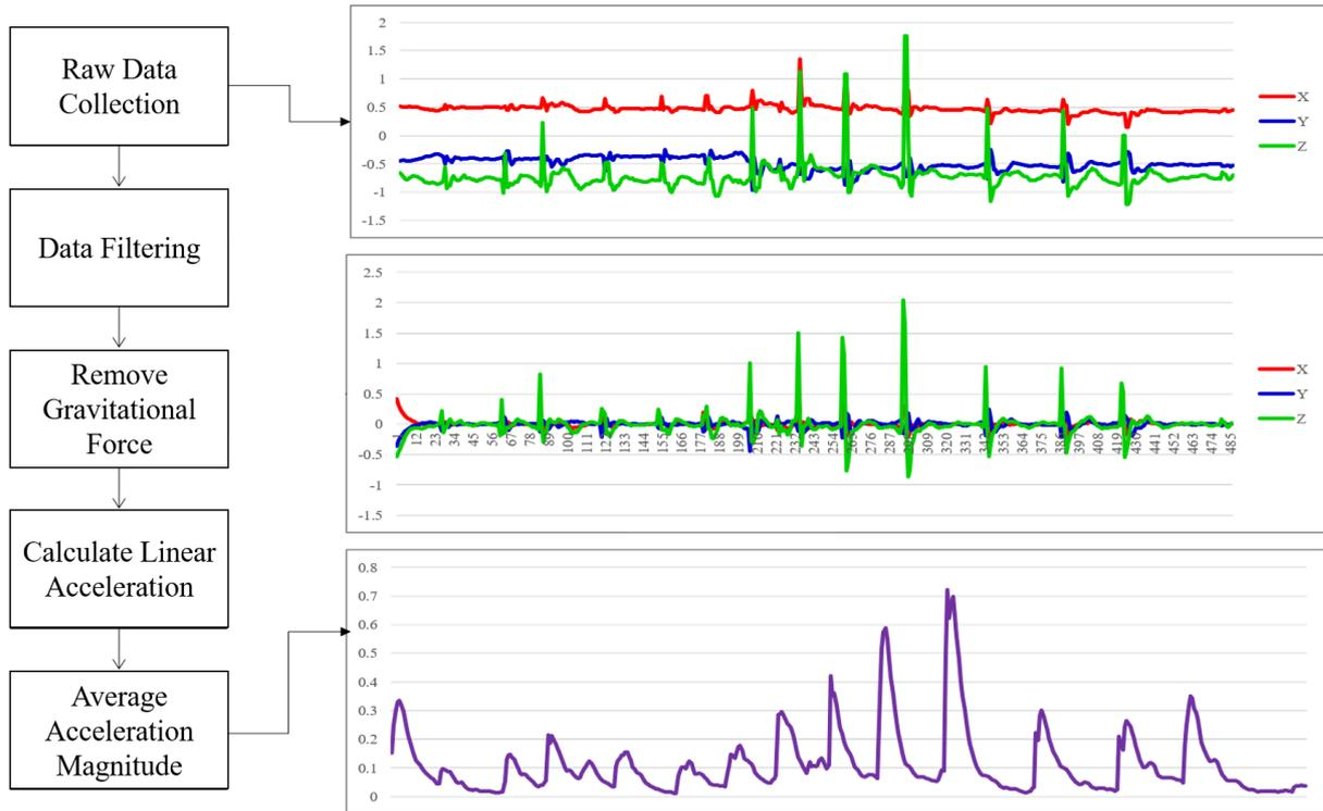
Fig. 3: Overall Procedure of Filtering Tri-Axial Accelerometer Sample
