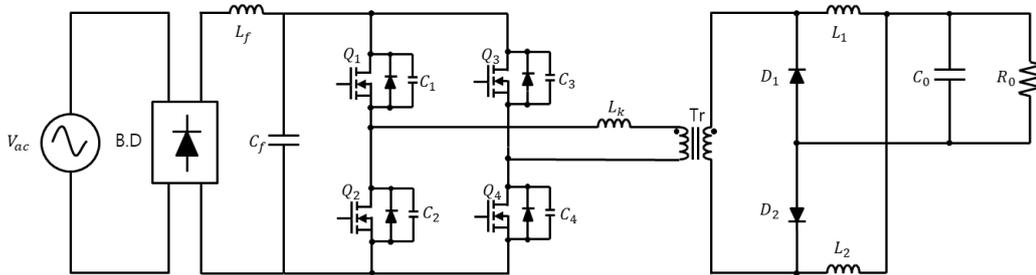
Figure 1: Circuit structure of 3kW DC-DC converter
