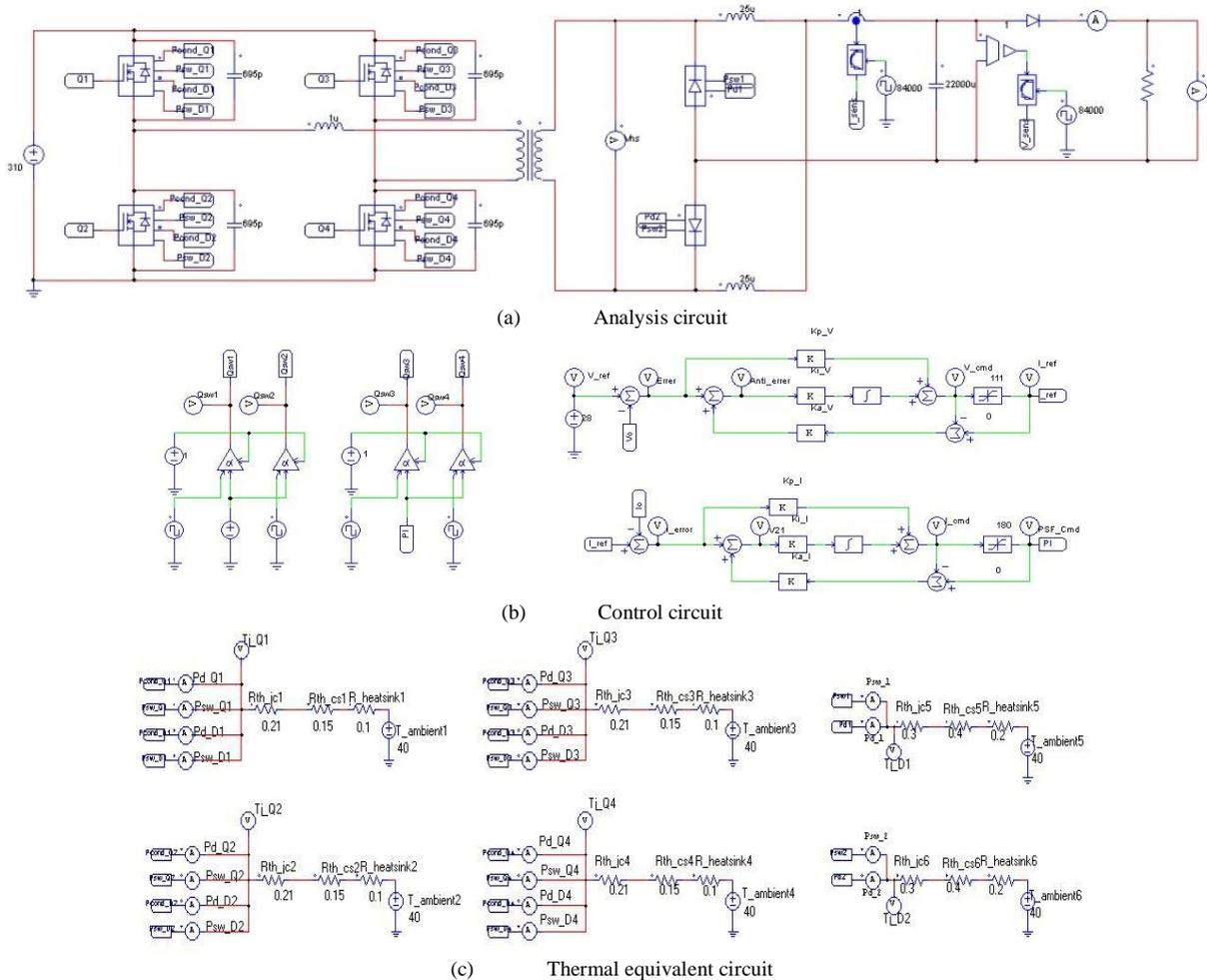
Figure 4: DC-DC converter analysis circuit
