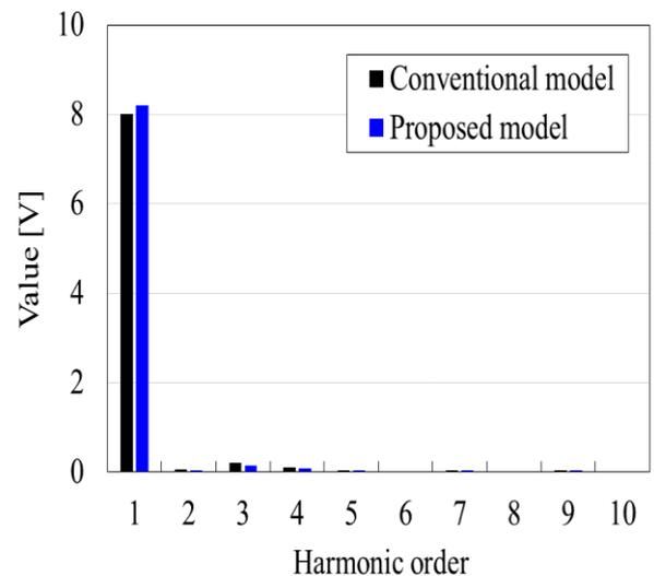
**Figure 7:** Comparison of the THD characteristics of the back-EMF
