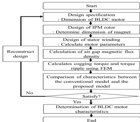
Figure 4: Proposed design algorithm of the BLDC motor for an EWP
