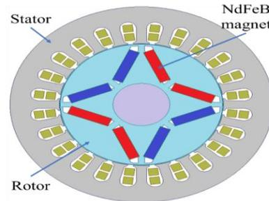
Figure 3: Cross section of an IPM BLDC motor (Conventional model)
