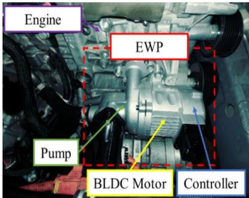
Figure 1: Structure of the EWP mounted on an engine
