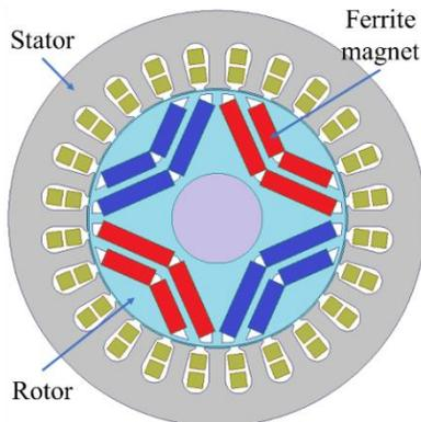
**Figure 5:** Proposed model of the IPM BLDC motor**Table 3:** Design parameter comparison of BLDC motors
