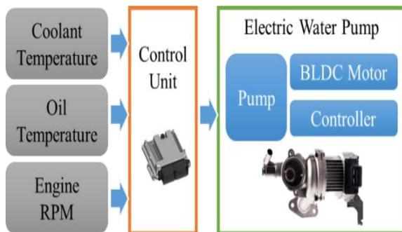
Figure 2: Overall structure of the EWP system
