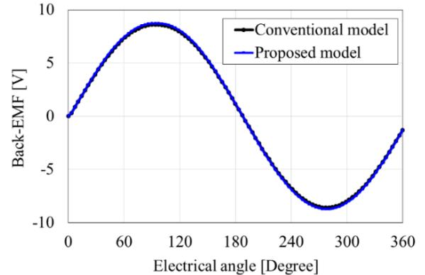
**Figure 6:** Comparison of the back-EMF characteristics
