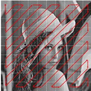
**Figure 1:** Illustrations of zigzag scanning order covering entire scope of an image data
