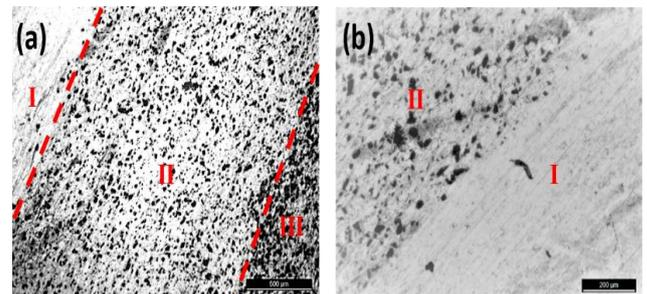
Fig.6: Microstructure of Al/ Al<sub>2</sub>O<sub>3</sub> FG sample observed under optical microscope
