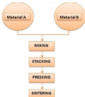
Fig. 3: Flow chart for Powder Metallurgy Process
