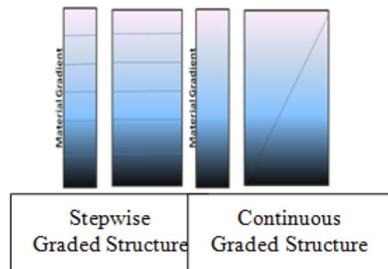
Fig.1: Schematic diagram of FGM
