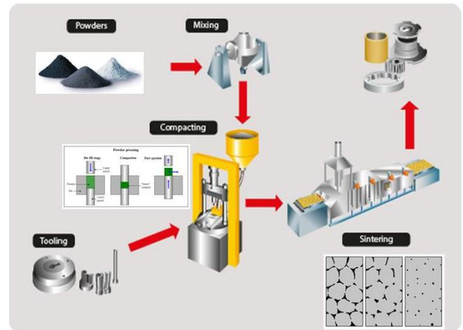
Fig. 4: Stages of Powder Metallurgy process
