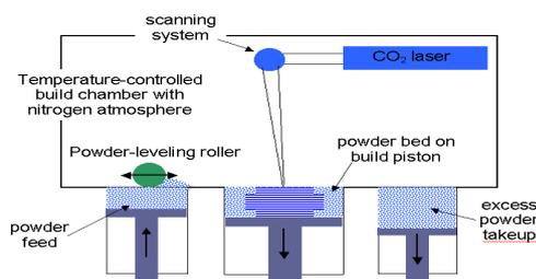
Fig. 9: Selective Laser Sintering Process
