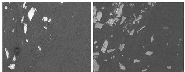
Fig.7: FESEM image of Al/ Al<sub>2</sub>O<sub>3</sub> FG sample showing different layers.
