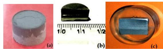
Fig.5: After compaction: (a) Raw FGM sample (b) Diameter of sample (c) Sample prepared for hardness test
