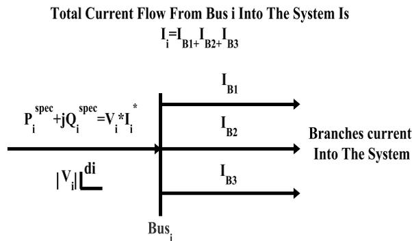
Fig. 1: Power Balance for Bus i.
