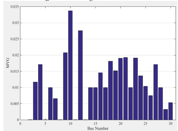
Fig. 4: MVG for Single DG and 0.1 P. U.
