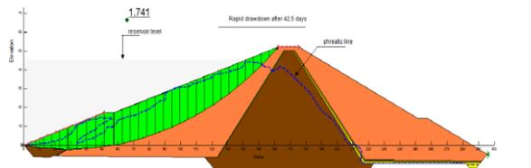
Fig. 10: Slip surface and factor of safety after 42.5 days when the dam is drawdown rapidly.
