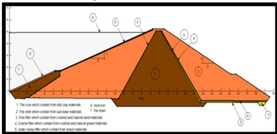
Fig. 1: Cross section of the dam
