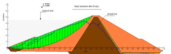
Fig. 11: Slip surface and factor of safety after 60 days when the dam is drawdown rapidly.
