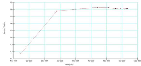
Fig. 8: Relationship between the factor of safety and the time for each upstream slip surface when the reservoir is drawdown rapidly.
