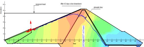
**Fig. 16:** Phreatic line, velocity vectors and flux suction quantity after 43 days slow drawdown.
