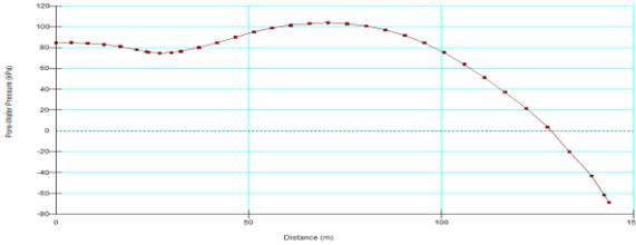
**Fig. 14:** Pore water pressure across the slip surface after (60 days).
