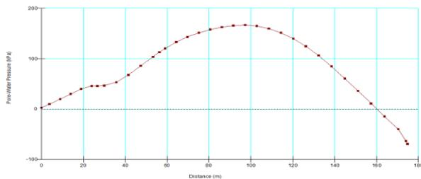
Fig. 5: Pore water pressure across the slip surface after (60 days) rapid drawdown
