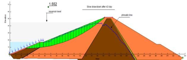
**Fig. 20:** Slip surface and factor of safety after 43 days when the dam is drawdown slowly.
