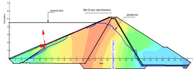
Fig. 7: Phreatic line, velocity vectors and flux suction quantity after 20 days rapid drawdown
