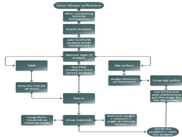
Fig. 2: SLOPE/W flow chart
