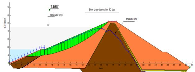
**Fig. 21:** Slip surface and factor of safety after 60 days when the dam is drawdown slowly.
