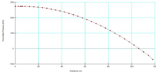
Fig. 4: Pore water pressures across the slip surface before the initiation of rapid drawdown condition
