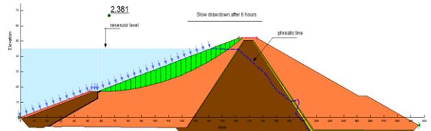
**Fig. 19:** Slip surface and factor of safety after 6 hours when the dam is drawdown slowly.
