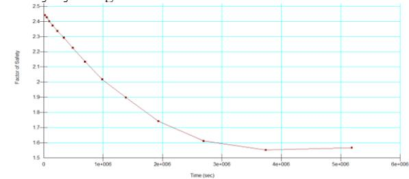
**Fig.18:** Relationship between the factor of safety and the time for each upstream slip surface when the reservoir is drawdown slowly.
