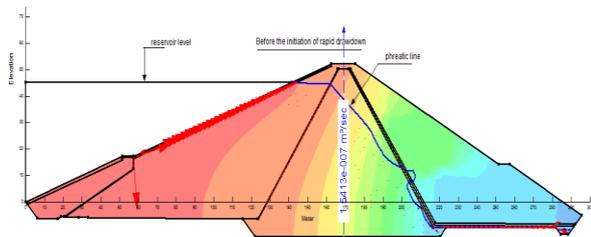
Fig. 6: Phreatic line, velocity vectors and flux suction quantity before the initiation of rapid drawdown
