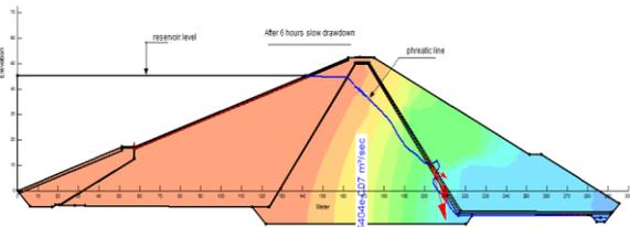
**Fig.15:** Phreatic line, velocity vectors and flux suction quantity after 6 hours slow drawdown.
