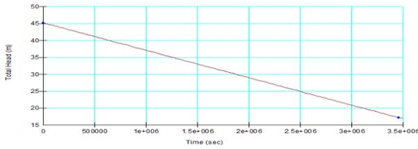
**Fig. 12:** Relationship between the total head and the time required to empty the reservoir by the slow drawdown
