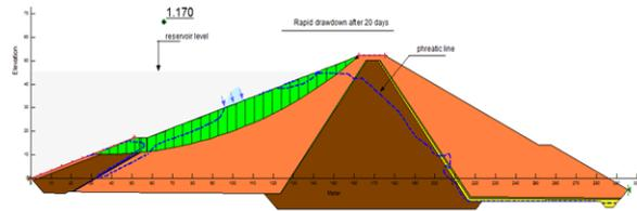
Fig. 9: Slip surface and factor of safety after 20 days when the dam is drawdown rapidly.
