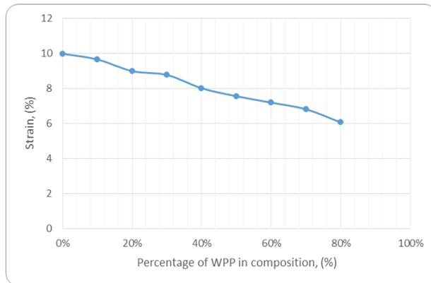
Fig. 4: Graph of strain versus WPC composition
