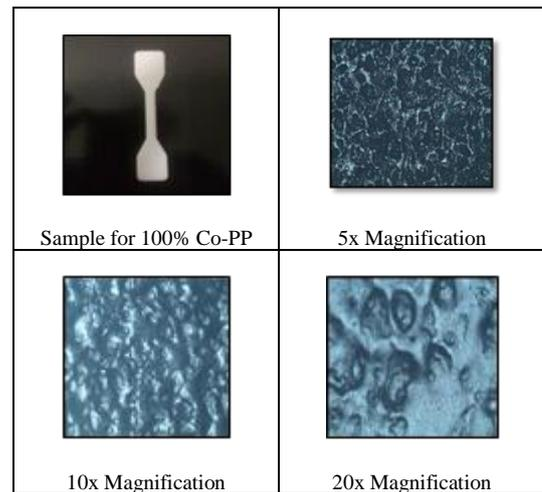
**Fig. 1:** Morphological view of 100% CO-PP from optical microscope
